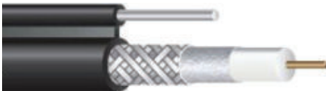
RG11-OB-90 RG11 Cable, Coverage 90%, Braid Shield aluminum 0.16mm x 168 wire, Messenger
