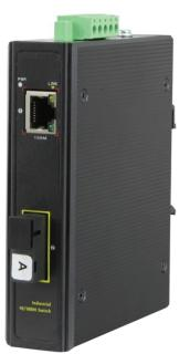
The IMC-FWXX-SC-20 is a 10/100M industrial Ethernet fiber switch independently developed by Focomm. It is designed to meet industrial fields and systems and can operate stably for a long time in harsh environments. It has 1\*10/100M RJ45 port and 1\*155M uplink SC port. Each port can support full line-rate forwarding.
