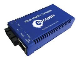
Media convector used for the exchanging between Ethernet and fiber. The machine comprises 1 Ethernet port and 2 fiber port, and expanded the LAN cable transmission distance from 100 meters to 20 kilometers. It realized the inter connections between different telecom equipment and widely been used in Telecommunication, CATV, Bandwidth network, CCTV where demands high performance and reliability network environment.
