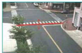
Trip wire Setting Line and detect direction in-out
